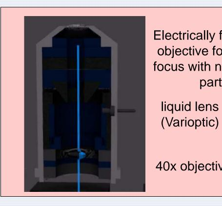
Electrically focusable objective for auto zfocus with no moving parts liquid lens
