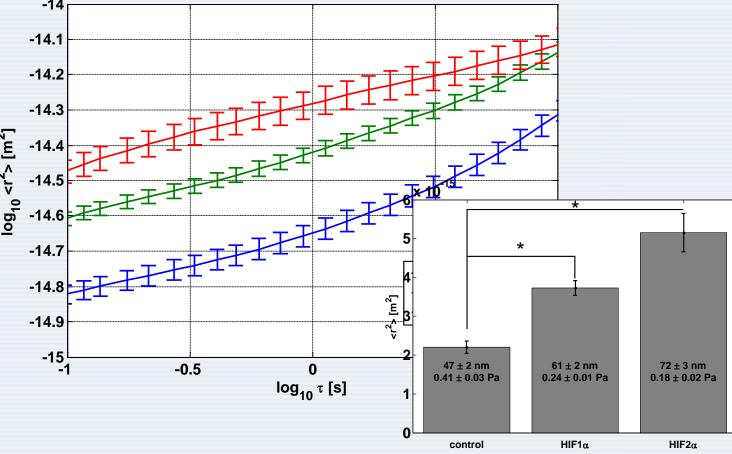
Average MSD curves for cell type. Each MSD curve above is a collection of 100s (melanoma) of beads. The bar plots represent average MSD at the 1-second time lag, the maximum timescale in which Brownian motion is the primary contribution to the motion of the bead. Error bars = SEM. \*P < 0.0001.
