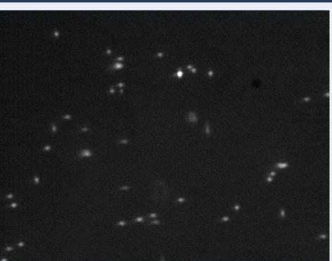
2 um fluorescent beads coated with fibronectin target attachment to integrins. Integrins receptors connect directly to the cytoskeleton of the cell allowing mechanical properties of the cells to be determined from the thermal motion of the bound beads.
