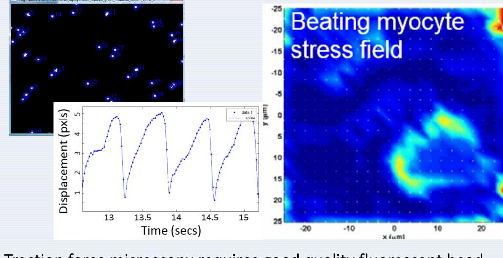
Traction force microscopy requires good quality fluorescent bead images at appropriate frame rates. We have demonstrated tracking of labeled beads at 40fps, 5 msec exposure times. We are working with the group of Prof. Jeff Fredberg at Harvard in incorporating their TFM code into the pipeline for the Panoptes instrument.
